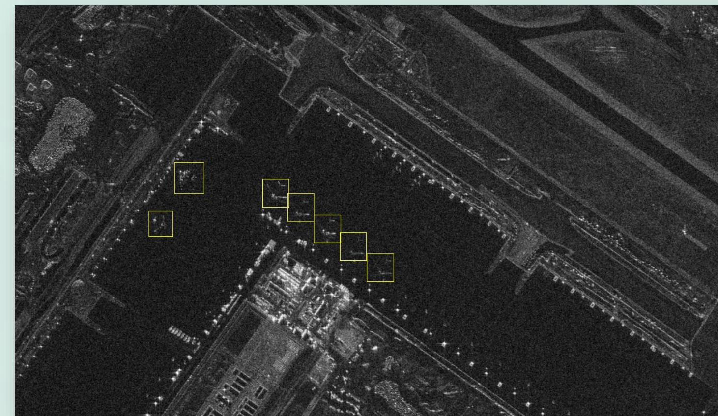
ICEYE Use of AI for SAR image for on-board object detection and classification
