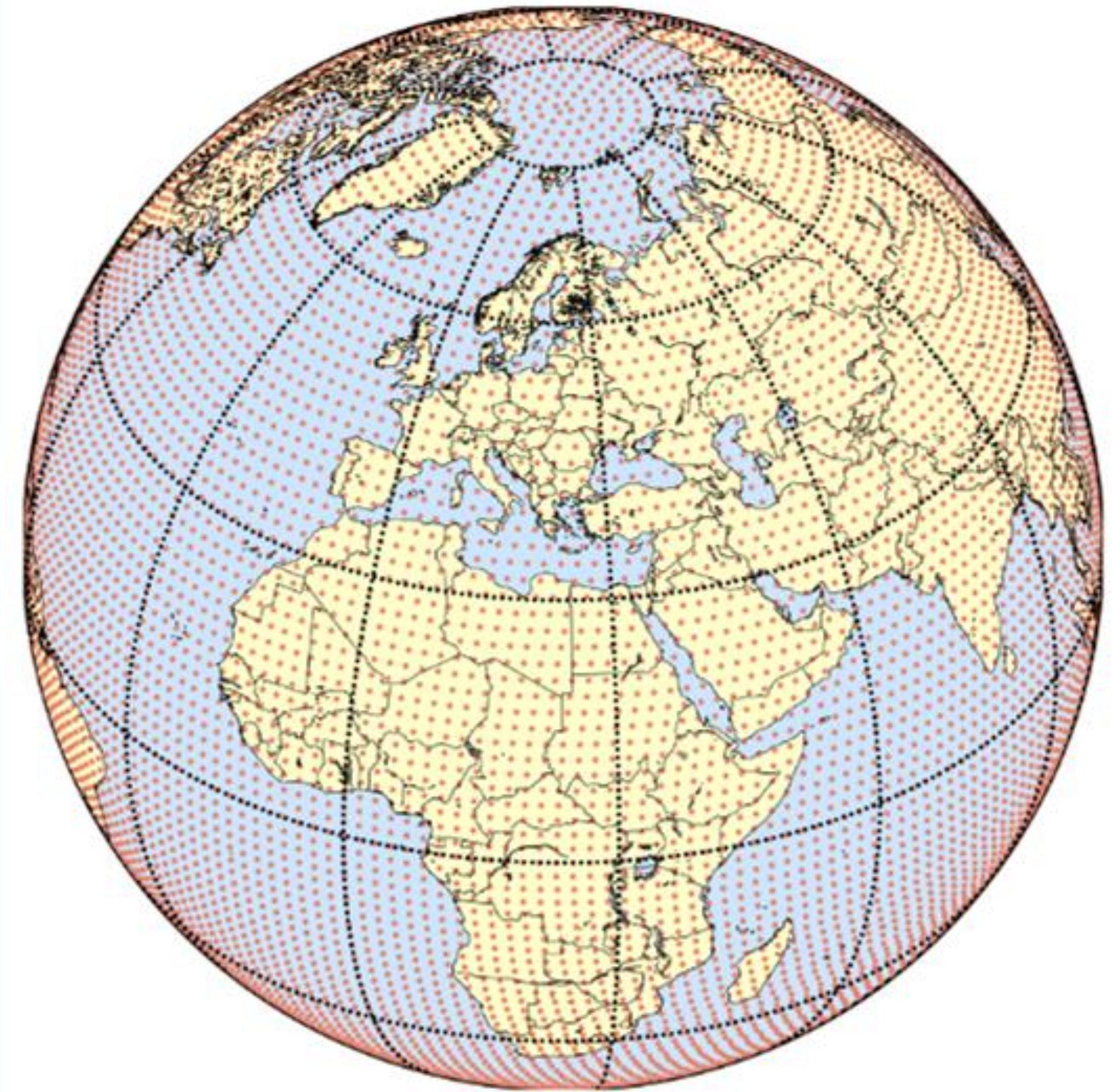
Major TOM's grid system. Each grid point gets a sample of data. 200km grid visualised, real data in 10km grid.
