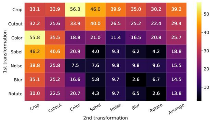
Figure 5. Linear evaluation (ImageNet top-1 accuracy) under individual or composition of data augmentations, applied only to one branch. For all columns but the last, diagonal entries correspond to single transformation, and off-diagonals correspond to composition of two transformations (applied sequentially). The last column reflects the average over the row.
